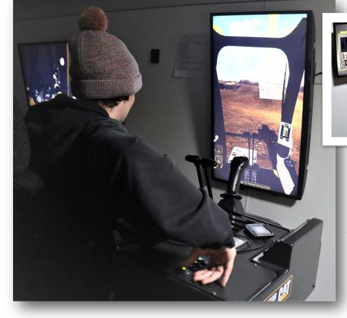
Heavy equipment simulators provide life-like sounds from the roar of a diesel engine to back-up warning signals and even vibrate so operators get an almost real learning opportunity. After a week of work on the simulators, students at the Linn Benton Detention Center will sprend a week operating real machinery.
